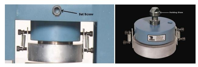
Figure 1 - Set Screw and Holding Stem locations
