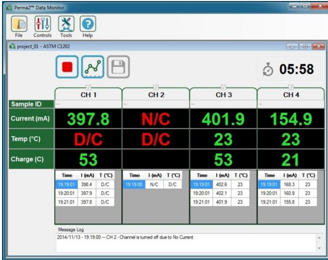
ASTM C 1202 Test Running
